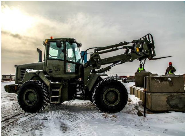
The MWT moves representative bridge concrete blocks
